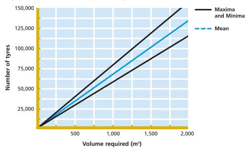
Figure 3 – Number of compressed tyres per cubic metre
