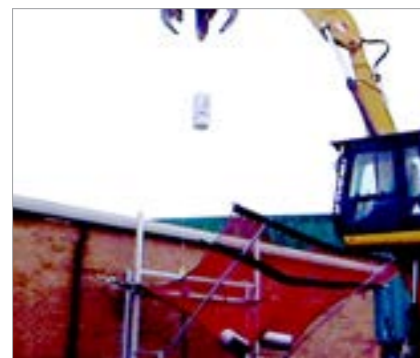
The Rapid-Net holding 2 100kg weights, about to catch a 3rd.
