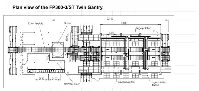
With a large and variable work space the area gantry robot is ideal for commissioning tasks. The diagram above shows how the robot can process twelve different orders simultaneously.
