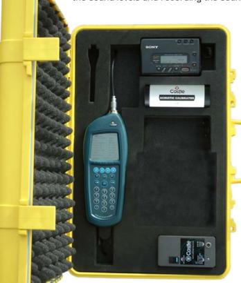
Having said that, the elements of the kit can also be used separately giving you the use of a powerful hand-held sound meter for multiple applications. As the case and connectors are weatherproof, it is also possible to use the kit for outdoor monitoring, be it a short or long term requirement.
