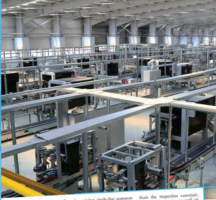
and non-round containers. Built on Bucher Emhart Glass' proven FleXinspect electronics platform, it also lets users add more inspection elements as and when they're required - for example, bringing in additional vision technologies to control finish and base quality.
