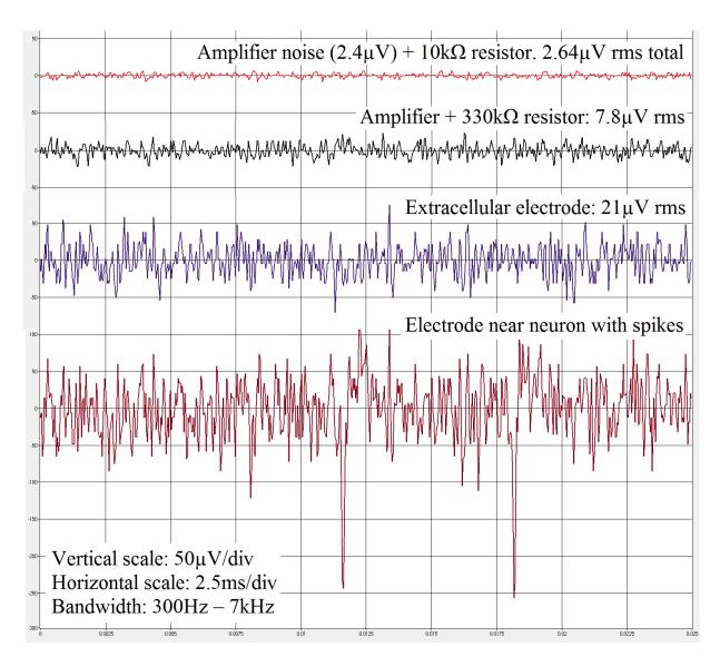
The uppermost waveform was measured when the neural recorder was connected to a  $10k\Omega$  resistor instead of the electrode assembly. The measured signal essentially represents the input noise of the preamplifier. The observed  $2.64\mu V$  rms noise is due to the  $2.4\mu V$  rms noise of the preamplifier and the uncorrelated  $1.07\mu V$  rms Johnson noise of the  $10k\Omega$  resistor.
