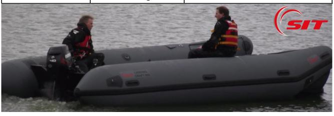
Hull material: Hypalon Drop-thread Weight: 144 KG
