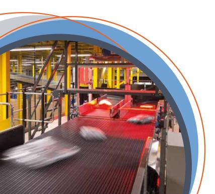
Installation of the new Interroll horizontal cross belt sorter and Intralox ARB diverters has enabled ASOS to double its throughput capacity whilst also increasing flexibility and resilience. Now parcels can be routed from the packing lines to either the new or existing sorters. This principle ensures there are no potential bottlenecks in the system, parcels and poly bags are in constant flow from pack bench to carrier trailer.
