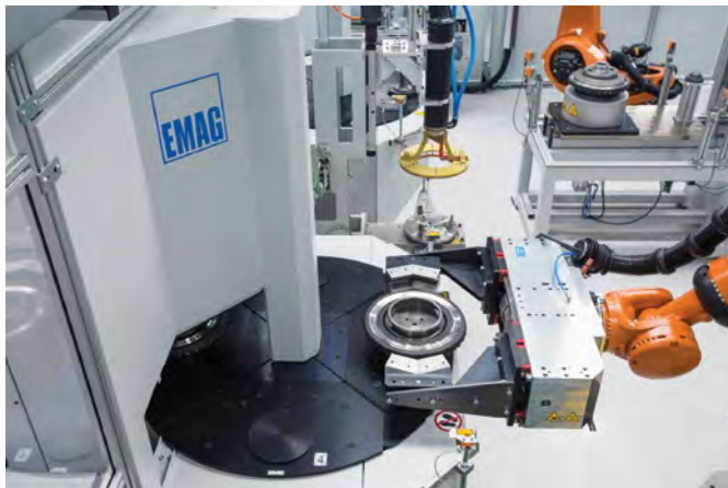
Housing parts, such as ring gears, are cleaned on the newly developed EMAG laser cleaning machine in preparation for the machining operation.
