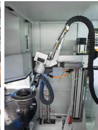
Housing parts, such as ring gears, are cleaned on the newly developed EMAG laser cleaning machine in preparation for the machining operation.
