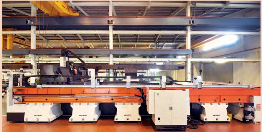
The gantry machining centre KMC-G is designed for workpieces from the aviation and machine tool industry. The x-axis of the travels over 13 metres
