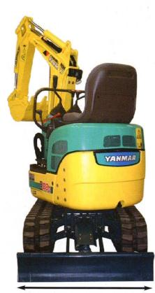
Unique machine of its weight class to go through openings of 700 mm.
