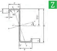
Note: Purlins are made from high tensile steel to be fastened rather than welded. Purlins can be ordered pre-cut to length and with pre-punched holes or slots.
