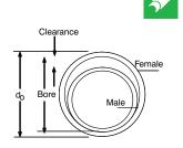
**Note:** Clearance = (AS/NZS 1163 Min do - 2t) - (AS/NZS 1163 Max do).
