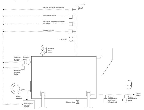
**Note:** For detailed requirements to suit different boiler types (eg steam cushioned) refer to BS EN 12953 Part 6 and SAFed PSG3 – Guidelines for the Operation of Hot Water Boilers. Solid fuels may require additional emergency cooling systems.
