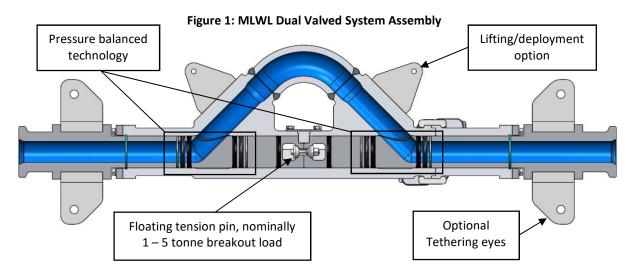
Secc's MLWL employs a floated tension pin mounted outside of the flow path. Floating the tension pin protects it from bending and torsional loads generated during operation. Being outside of the flow path protects the pin from forces generated from flow or pressure fluctuations.
