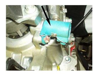
Locate blanking plug, remove and install sender unit supplied
