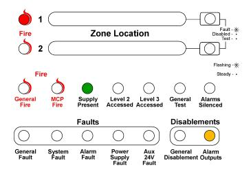
Figure 10.1. Example of the display when disabling the alarm outputs.
