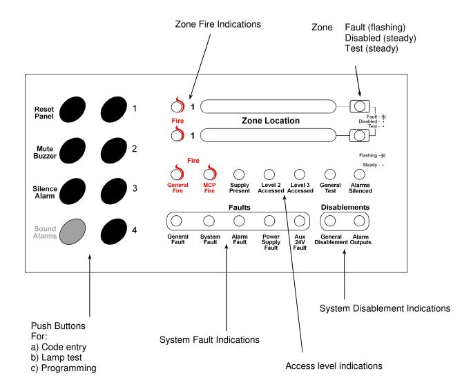
Figure 5.0 Front panel Indications and controls
