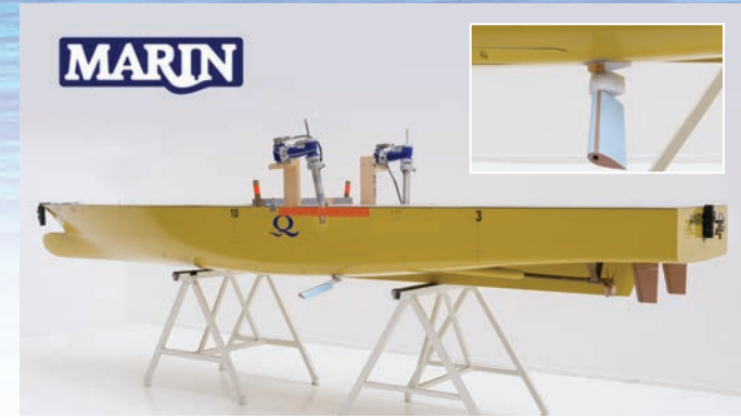
Above: A precision built model was used for both underway and Zero Speed™ tank testing.
