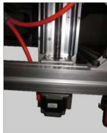
Lifting controlled by screw and stepper motor
