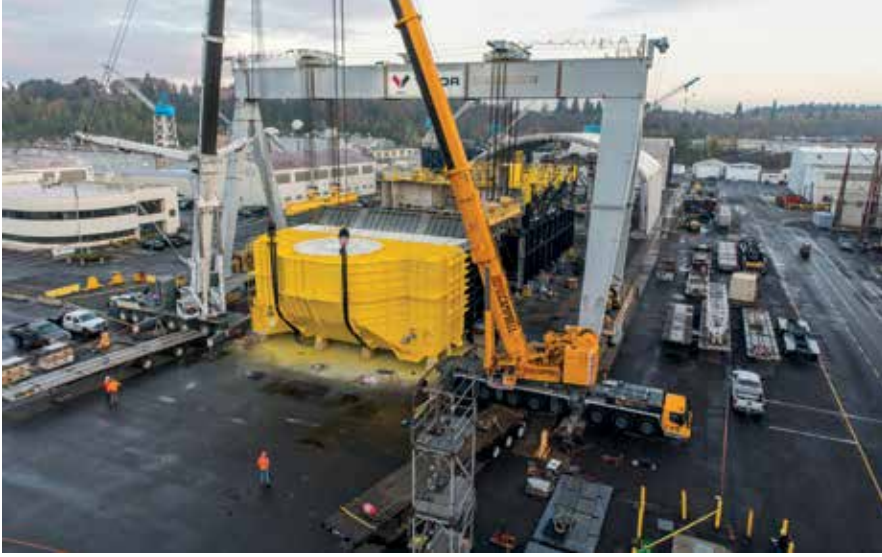
The 826-ton Ocean Energy Buoy measures 125 by 59 feet, with a draft of 31 feet, and has a potential rated capacity of up to 1.25 MW in electrical power production.
