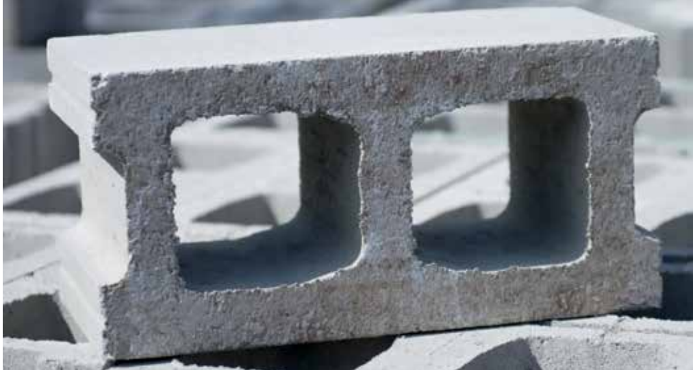
A cinder block injected with carbon PHOTO COURTESY CARBONCURE
