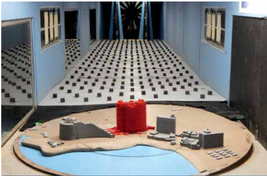
A scale model of Guam's new luxury Tsubaki Tower (red) in BASE's wind tunnel PHOTO COURTESY BALDRIDGE & ASSOCIATES STRUCTURAL ENGINEERING INC.
