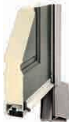
Wheelchair Access Threshold MDS25/5/2 (15mm) Distance from bottom of door leaf to bottom of threshold 18mm
