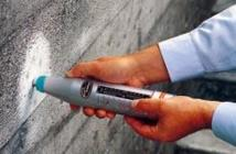
Original Schmidt Concrete Test Hammer
