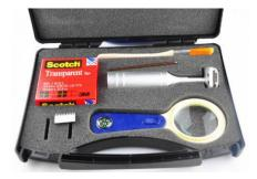
The round cutting knife of the Cross Cut Adhesion Tester Kit has eight cutting edges that can be changed easily by rotating the knife, the self-positioning knife bracket ensures equal pressure on the cutting knife.
