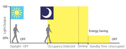
We achieve this using the latest motion sensor technology combined with step-dim ballasts in our Lumisaver system, or standard HF ballast in our Energysaver system.
