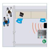
Once that particular instance has finished the data logger will continue to take readings but only log when presence is detected
