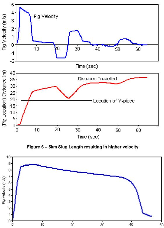
Figure 5 – 3km Gas Slug resulting in pig reversal
