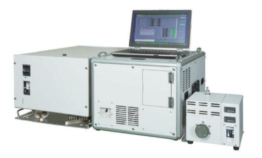
The A&D BOB-1000FT multi-component analyzer system has been designed for the continuous measurement of undiluted vehicle exhaust under real world conditions.
