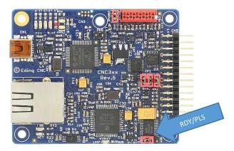
This jumper is used to set the output signal that is present on the I/O pin 'WATCHDOG/SYSRDY'.
