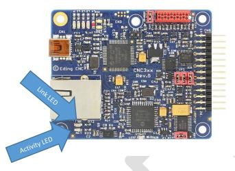
The LINK LED indicates if a network cable is connected. The ACTIVITY LED will blink if there is network communication.
