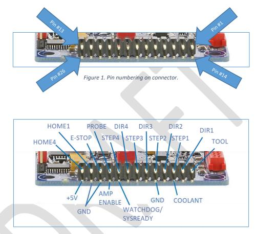
Figure 2. Functions on connector overview.
