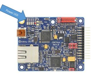
This blue power led indicates when power is applied to the board.
