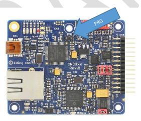
If this jumper is place the board will skip the bootloader mode and will go directly to starting the firmware.
