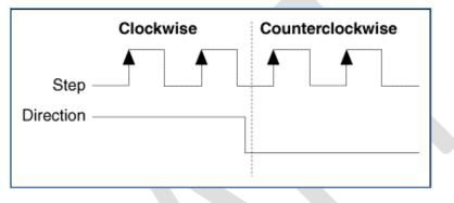
Figure 8. Example of STEP/DIRECTION signal.
