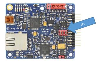
This jumper can be used to deactivate the signals on some I/O pins. Currently make sure that all jumpers are mounted.
