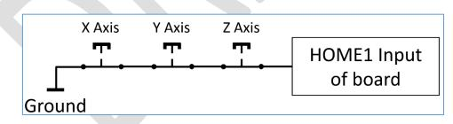
Figure 17. Connecting Normal-Closed home switches in series.
