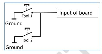
Figure 13. Connecting multiple tools to probe input.
