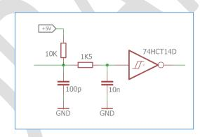
Figure 14.E-STOP input circuit.
