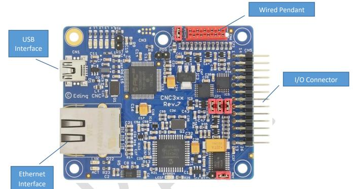
The purpose of the board is to offer a simple controller that can be used for operating small CNC machines that need only limited I/O.
