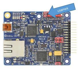
This jumper is used to power the board via the USB interface. The board can also be powered through an external pin.
