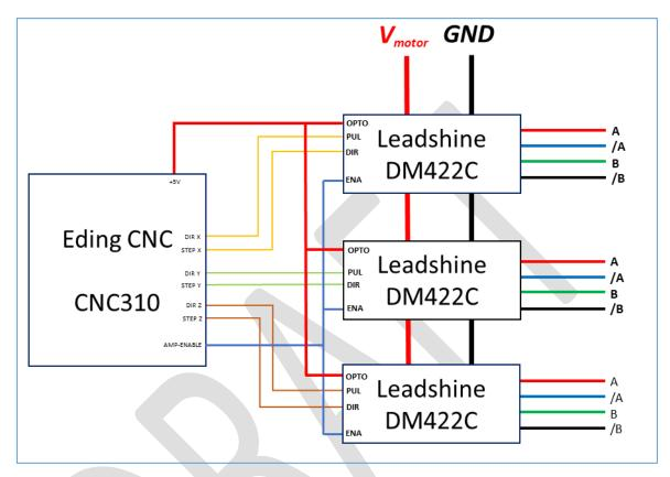
Figure 21. Connecting CNC310 to Leadshine DM422C.
