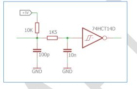
Figure 11. Probe input circuit.
