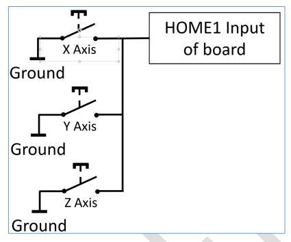
Figure 18. Connecting Normal-Open home switches in parallel.
