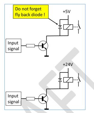
Figure 6. How to switch a power relay.
