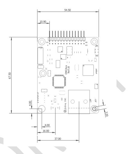
The controller can simply be connected by using standard connector (2x13 pole), pitch 2.54mm/0.1":
