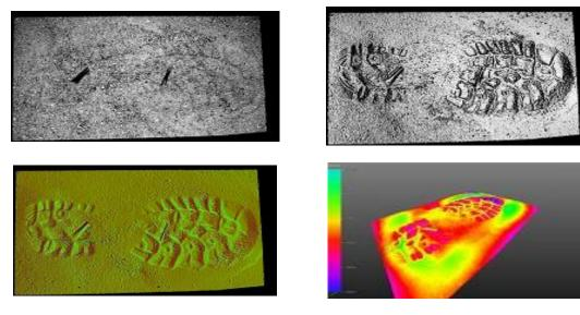
Fig. 5: Impressions of 3D-Forensics analysis software: raw data scan (top left), improved impression visualisation (top right and bottom left), 3D view with depth real-time analysis (bottom right)
