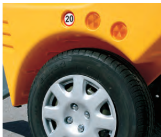
Integrally moulded mudguards
