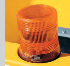
Amber flashing light
