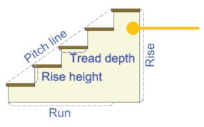
A typical staircase and terms used to describe the various sections.
