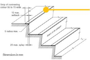
A typical stair nosing profile with nosing strip as in AS1428.1.
