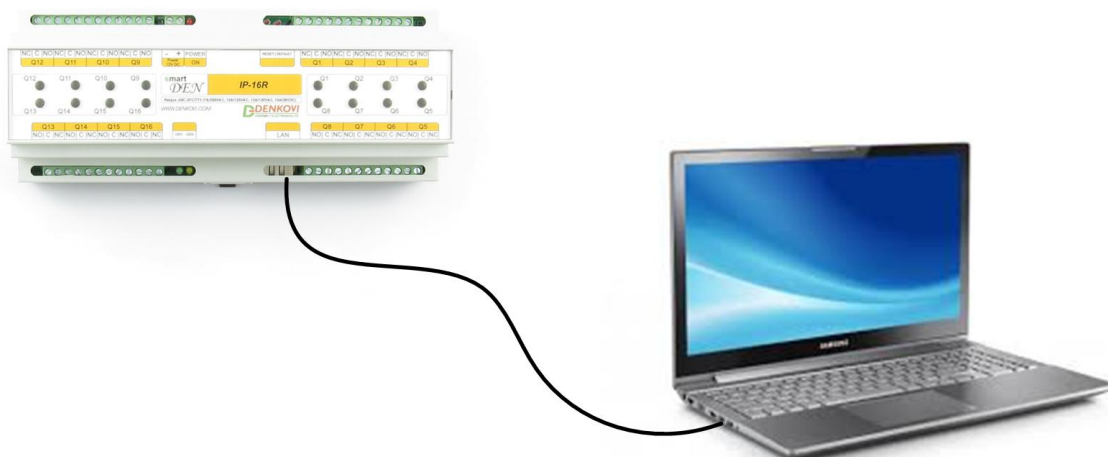
Figure 6. Connecting SmartDen IP-16R to a computer directly. This is the recommend initial connection.
