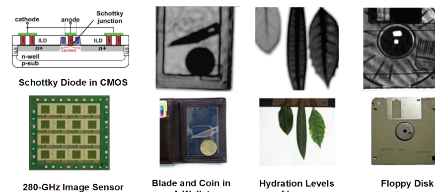
Figure 3. Using a terahertz CMOS image sensor based on Schottky diode, we performed active imaging for various objects [R. Han, et al, ISSCC 2013].
