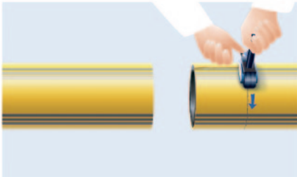
Fig. 2.14 Removal of the protective coating with the egeplast M10 peeling tool
