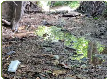
Flow logger in Dry Streambed Awaiting a Storm to Log Flow Data
