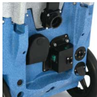
Slide-in 2.8 kw heater
