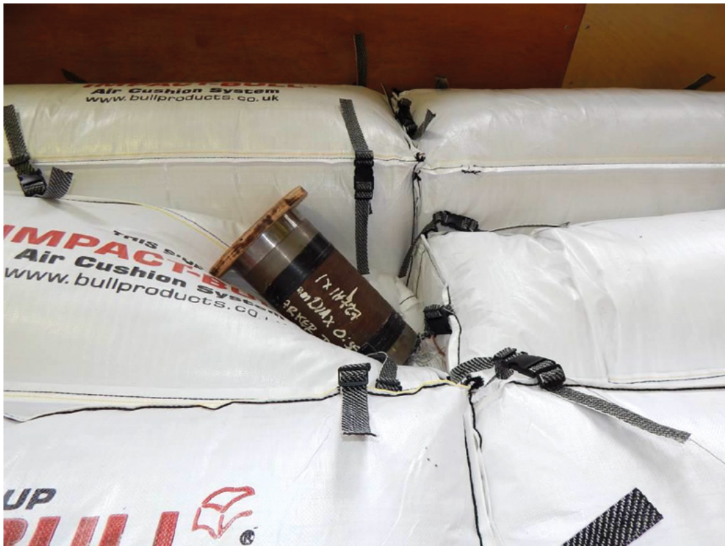
Figure 3 View of the bags after an impact
