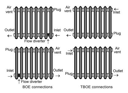
For installations with BOE connections, a flow diverter should be fitted at the inlet connection for radiators up to 20 sections long. The flow diverter is attached to the inlet bush connection and is supplied as an accessory. The vent valve should always be fitted at the outlet end of the radiator. If necessary, rotate the radiator to position the vent correctly.
