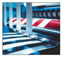
efficiently an adhesive will die-cut. In the case of double-faced spacer tapes used in diagnostic test strips, it is the interaction of the adhesive, substrate and bonded layers that ultimately determine die-cutting performance.
