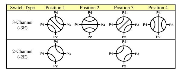
Figure 1: Precision Waveguide Switch Rotor Positions
